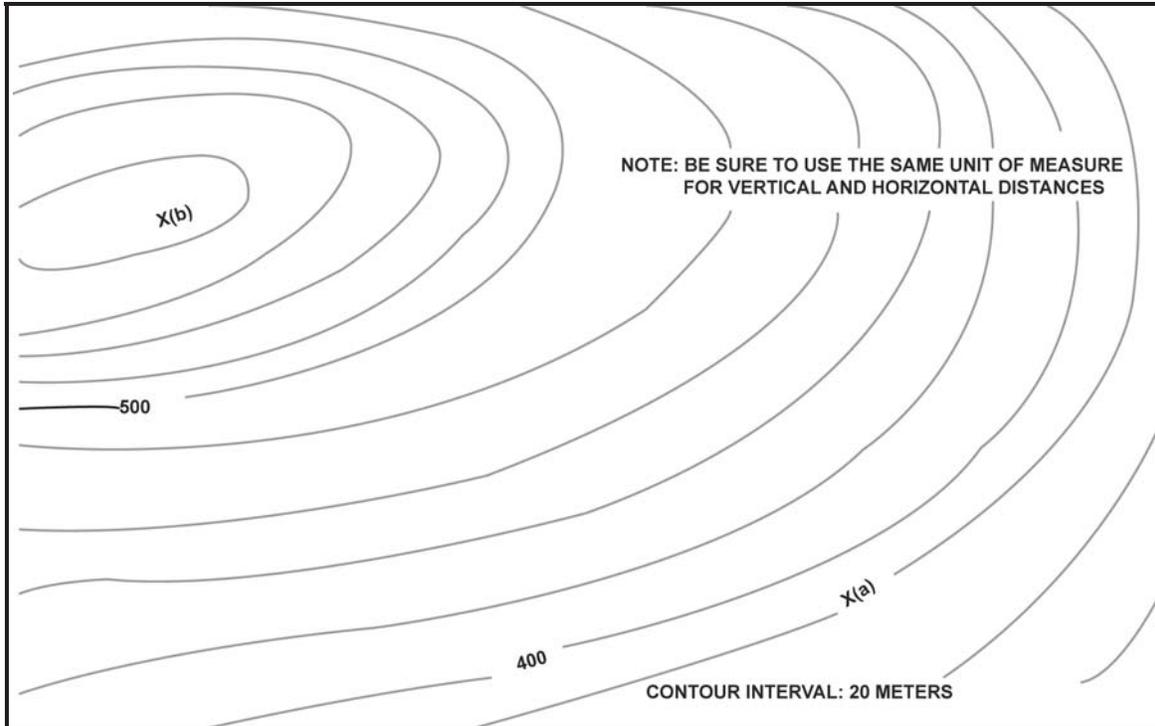
**Figure 9-10. Contour lines around a slope**
