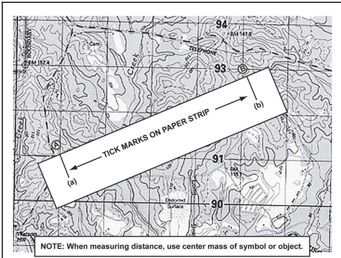
**Figure 5-3. Transferring map distance to a paper strip**
