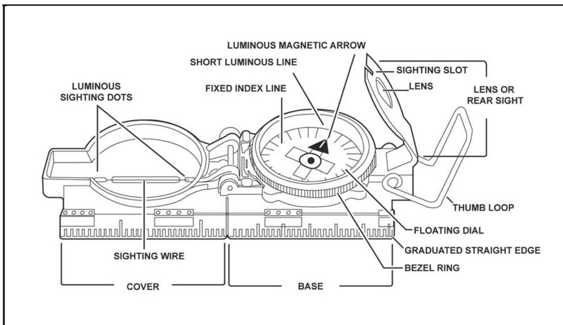
**Figure 8-1. Lensatic compass**
