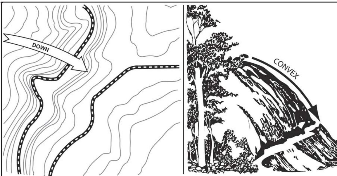
Figure 9-8. Convex slope
