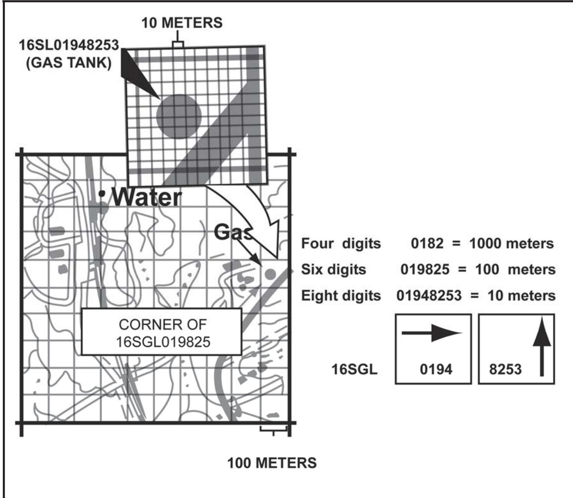
Figure 4-22. The 100-meter and 10-meter grid squares
