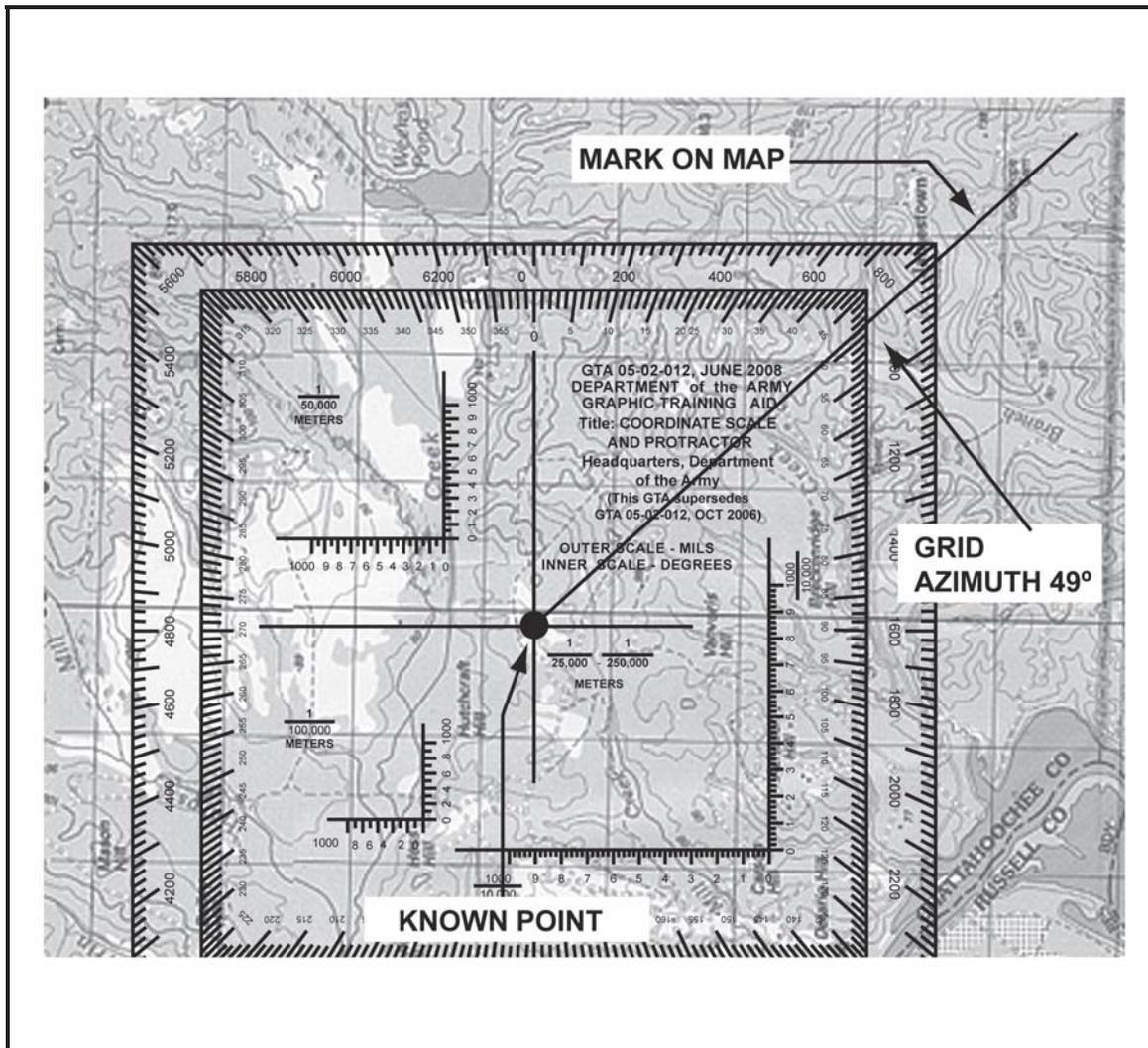
Figure 6-7. Plotting an azimuth on the map
