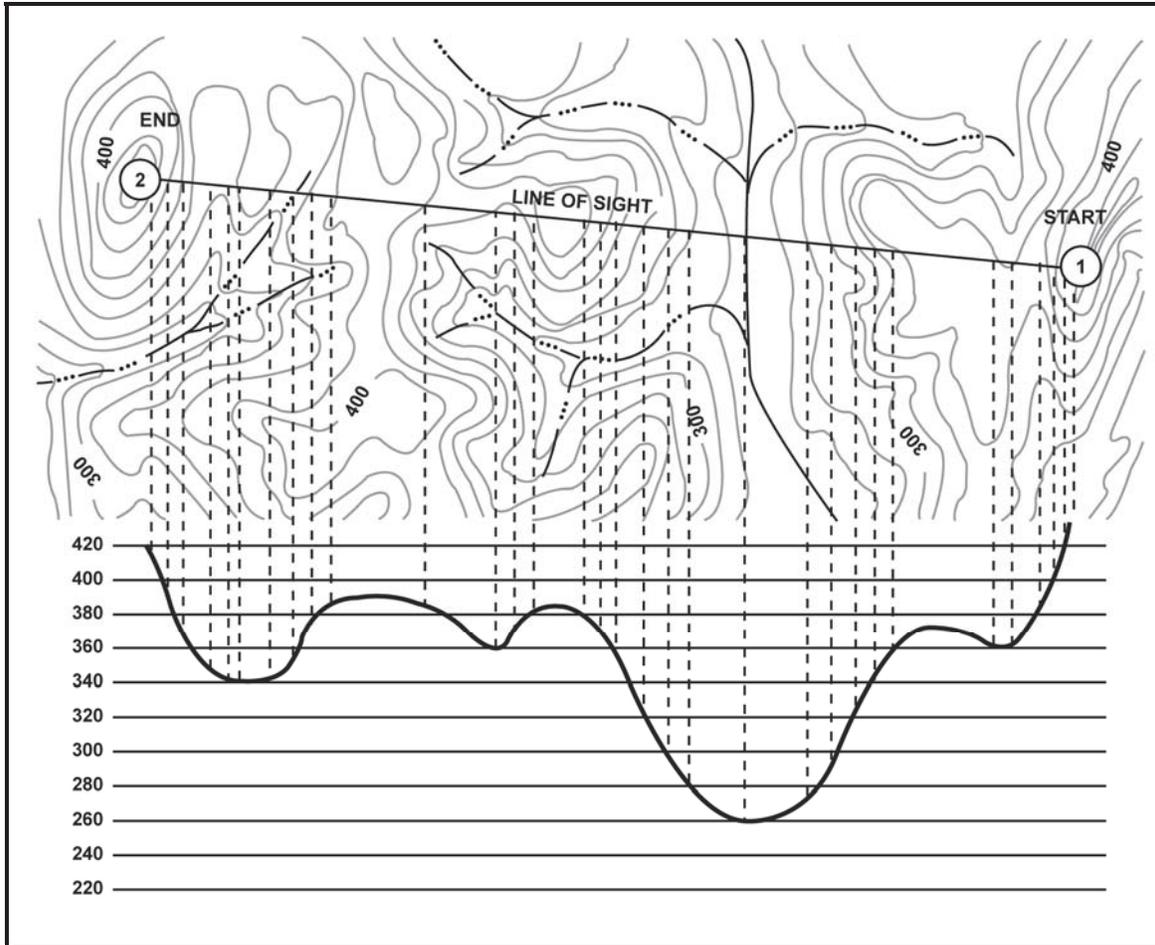
**Figure 9-28. Dropping perpendiculars**
