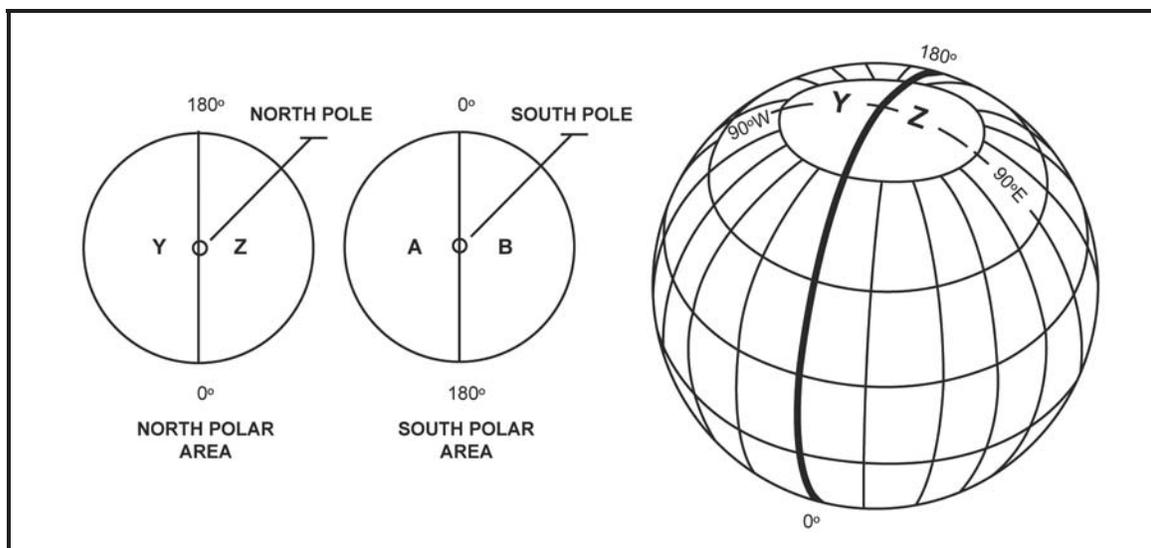
Figure 4-12. Grid zone designation for UPS grid
